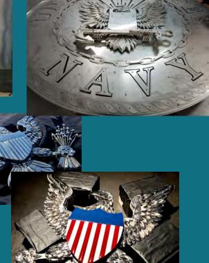
All pieces for the various Seals on America's Wall of Honor are cut from 5' x 10' sheets of stainless steel. Since each Seal required hundreds of pieces, each required up to 10 sheets of steel.
